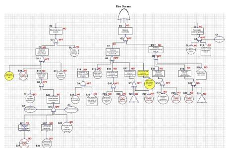
Figure 3: A Fault tree to illustrate how fire may occur in an electrical coffee maker for Project III
